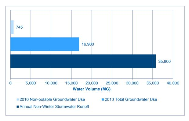
Chart 6. Comparison of Annual Groundwater Use by Identified High-Volume Non-Potable Water Users with Average Annual Stormwater Runoff and 2010 Groundwater Use within the Northwest Metro Study Area
