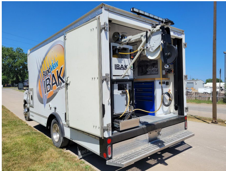
Crews control the camera inside the sewer pipes from a truck like this.
