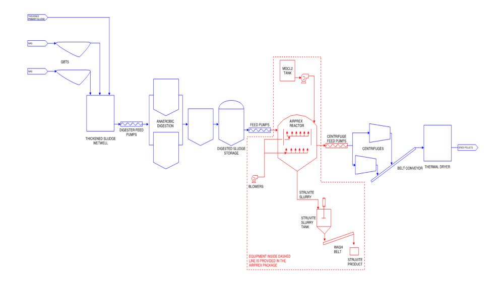
Figure 1-12: Blue Lake WWTP proposed flow diagram for phosphorus management approaches using biosolids harvesting/sequestration technologies.
