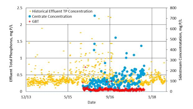
Figure 1-1: Blue Lake WWTP historical effluent and sidestream total phosphorus concentrations. Current permit limit is 1.0 mg P/L.
