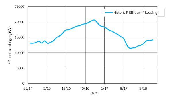
Figure 1-2: Blue Lake WWTP historical annual effluent total phosphorus loading. Current permit limit is 58,024 kg/yr.
