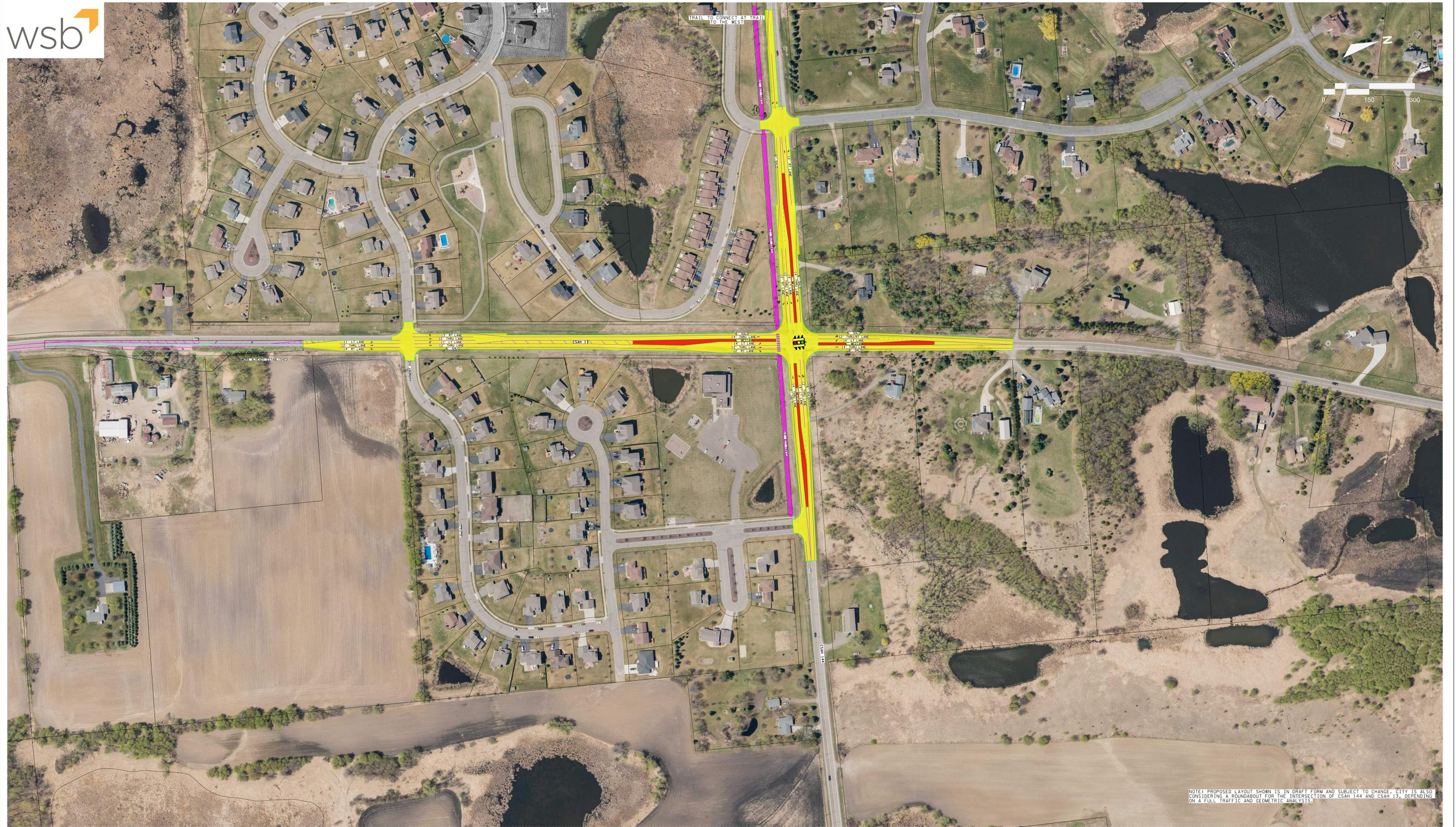
NOTE: PROPOSED LAYOUT SHOWN IS IN DRAFT FORM AND SUBJECT TO CHANGE. CITY IS ALSO CONSIDERING A ROUNDABOUT FOR THE INTERSECTION OF CSAH 144 AND CSAH 13, DEPENDING ON A FULL TRAFFIC AND GEOMETRIC ANALYSIS.
