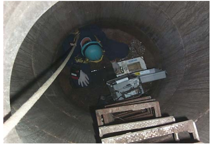
IWPP technician measuring wastewater flow coming from the city of Hopkins.
