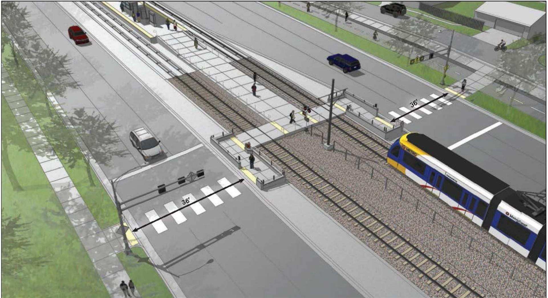
Figure 4-4. Provisions for a Cycle Track on the North Side of Olson Memorial Highway
