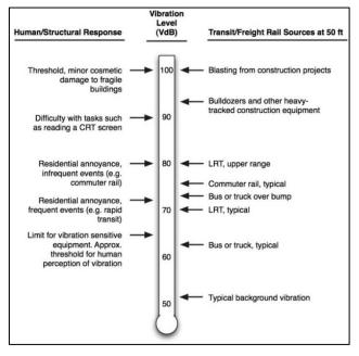
Ground-borne noise (GBN) is also assessed. GBN is a form of low-frequency noise that radiates from building walls and ceilings due to vibration caused by LRT or freight rail operation. Because airborne noise typically masks GBN for above ground (at-grade or elevated) transit systems, GBN is only assessed for operations in a tunnel (where airborne noise is not a factor) or near locations such as recording studios that are well insulated from airborne noise.
