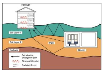
Vibration and GBN impact assessments are based on applicable FTA and Federal Railroad Administration (FRA) models, and are assessed using the source-path-receiver framework. Some of the key components of a vibration impact assessment include:
