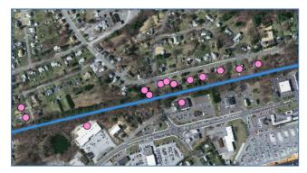
The output of a vibration or GBN impact assessment includes locations with vibration or GBN impact (purple). This information is used to determine the location and extent of any potential vibration mitigation.
