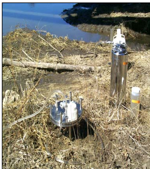
PCB Monitoring at the Minnesota River at Judson site. The picture on the left shows the pumping apparatus in the river. The picture on the right shows the filter apparatus and the sample collection bottle.
