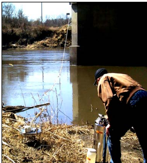
PCB Monitoring at the Minnesota River at Judson site. The picture on the left shows the pumping apparatus in the river. The picture on the right shows the filter apparatus and the sample collection bottle.
